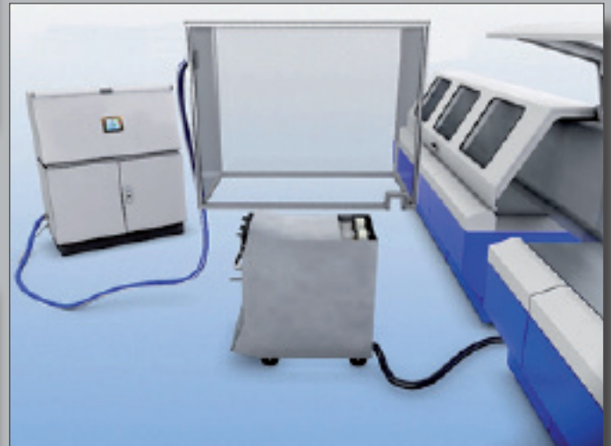
The dry-air box placed over the glue-trolley
